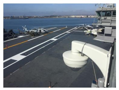
Working closely with Layer3, Bill McClurg also chose SD8364E, speed dome network cameras for the zoom capabilities in parking lot as well as ship deck monitoring and IP8155HP, box network cameras. VIVOTEK's SD8364E 1080p full resolution speed dome delivers superb image quality with its 30x optical zoom lens, perfect for monitoring wide open spaces. SD8364E's IP67 and NEMA 4X-rated housing protects against rain, dust and corrosion as well as operates under extreme weather conditions
